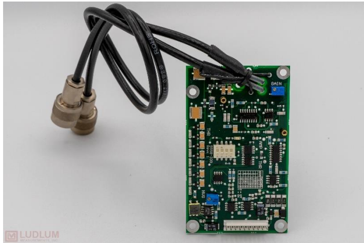
5558-339 : M 4525 SINGLE GAMMA PREAMP BOARD
