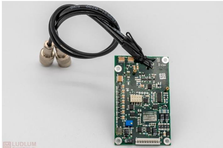
5558-344 : M 4525 DUAL GAMMA PREAMP BOARD
