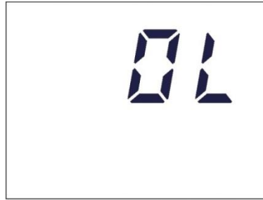
Figure 7: Detector Overload Alarm will also flash.
