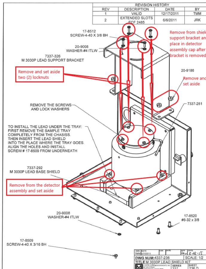
The assembly with the shield may be placed upside-down and the detector cleaned as described previously or as seen in the PIPS cleaning video. Re-assembly of the system entails reversing the above steps with the replacement of the detector back into the housing, as well as the replacement of the foam pucks and securing the assemblies back into place. The system should be powered up and checked for function prior to securing the cover.
