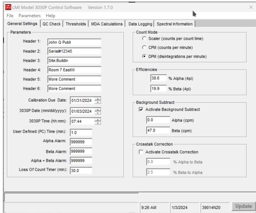
The following parameters require a password: Calibration Date, Date, Time, Background Subtract On/Off, Alpha Background Subtract, Beta Background Subtract, Alpha Efficiency, Beta Efficiency, Crosstalk On/Off, Alpha Crosstalk, and Beta Crosstalk.
