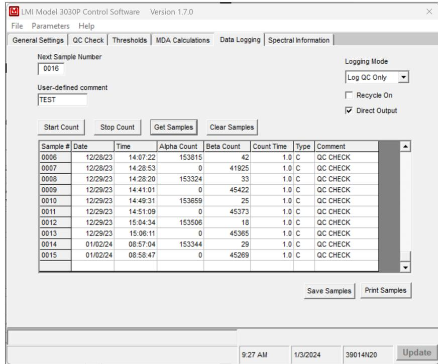
The Model 3030P can store 600 samples in its data logging memory. The following fields are stored with each sample: time, date, alpha reading, beta reading, count time, count mode, and user-defined comment.
