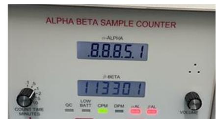
A 99:99:99 display with decimals between each “9” means that the instrument has exceeded its count/count rate capacity and is currently taking a count (shown below).
