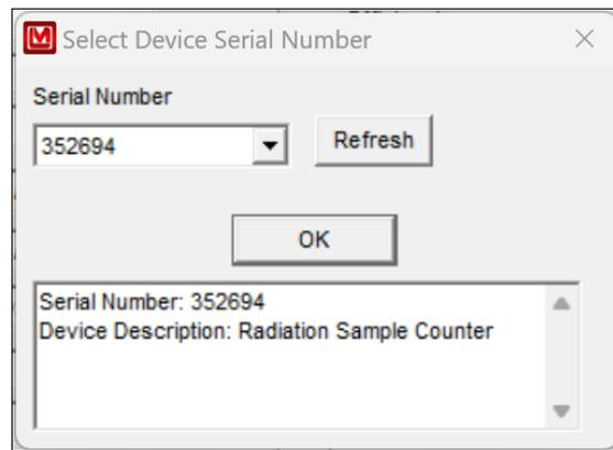
When the software is started, a dialog box is displayed allowing the user to select the instrument serial number from the drop-down list. The number of devices attached, their serial numbers, and the device descriptions are displayed in the text box. After a serial number is selected, the instrument's parameters are downloaded and the main screen is displayed.
