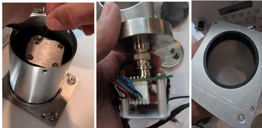
If the detector mounting and O-ring has contamination, an alternative and more extensive process of removing the entire cylindrical detector assembly and shield from the Model 3030P chassis can also be accomplished. Following the same steps above, power down and remove the cover of the Model 3030P and remove the connectors and the lead shield bracket.
