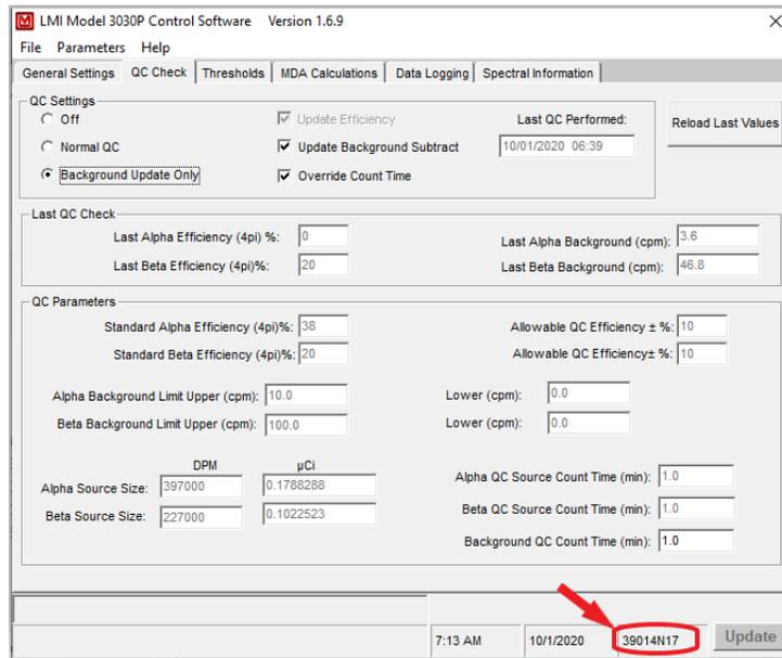
If using the computer interface, start the interface program from the appropriate directory/shortcut and set the desired operating parameters described in detail in Section 6 of this manual. Also, if desired, perform a QC check. See Section 6 of this manual for further details on QC check.
