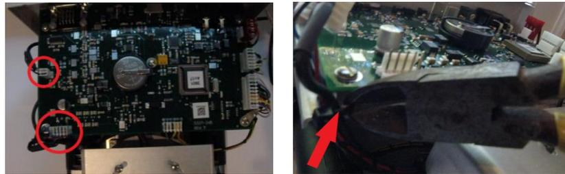
The connector assembly is wire-tied to the left bottom front support post of the circuit board (as viewed from the right photo above). Cut this wire tie and unplug the two connectors from the circuit board.
