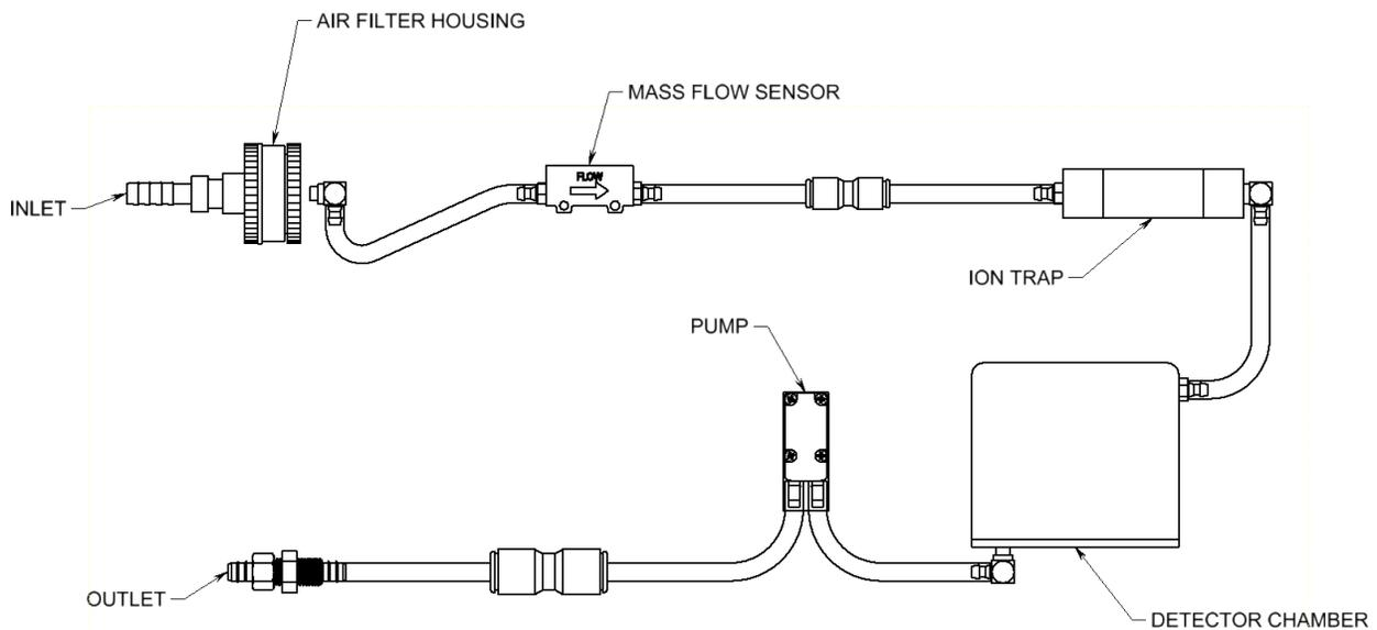
Figure 4-3. Air Flow Diagram.
