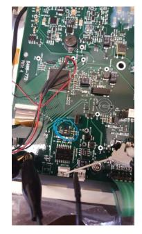
To enable RS-232 or Relay operations, open the battery compartment and remove the batteries from the Model 3276. Next, loosen the four captive pan-head screws that fasten the bottom cover. Gently remove the bottom cover of the instrument. The DIP (dual in-line position) switch should now be visible adjacent to the display ribbon cable.
